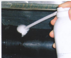
Apply foam to the area to be tested using the applicator.
